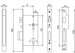
Technical drawings all measurements are in mm.
