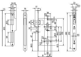
Technical drawings all measurements are in mm.
